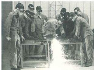
During a sixth hour Mr. Kitchens demonstrates the use of oxyacetylene cutting equipment to Farm Mechanics students.
